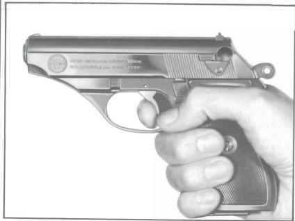
After the first shot has been fired the pistol functions semi-automatically, utilizing the recoil from each shot to push the slide rearward, extract the fired cartridge case from the chamber and eject it from the pistol through the ejection part. The rearward movement of the slide also cocks the hammer. The forward re-
