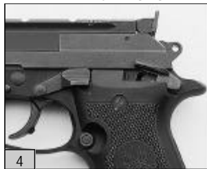
with hammer in half-cock position
