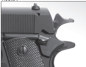
The hammer in the half-cock position.
