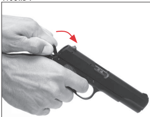
Lowering the hammer to the dropped position.
