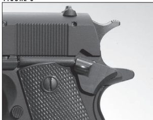
The hammer in the dropped position.
