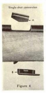
the movement of the breech bolt. Either .22 Short, Long, or Long Rifle cartridges may be dropped on the loading ramp and fed into the chamber by closing the breech bolt in conventional single shot fashion.
