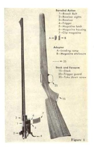
ger will pass through the opening in the stock into the trigger guard. Force is not required in fitting the two units together.
