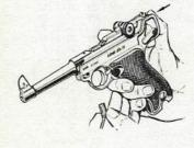
10. Pull the barrel forward against spring tension and at the same time insert the locking bolt.
