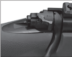
“Safety” shown in the off safe position.
