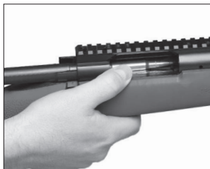
Press the cartridge down until it snaps into place.
