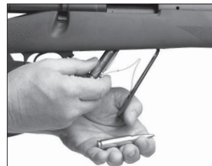
Catch the cartridges as the floorplate swings down.
