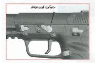
When the manual sofety is at the (raised) 'safe' position, the red marks are NOT visible
