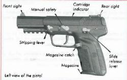
In convenional gun terminology, the position and movement of pistot parts are described as they occur with the pistot housantal and in normal firing position. The mustle is forward or front, the pistot grip is rearward or rear, the trigger is downward or underneath, the sights are upward or on top.
