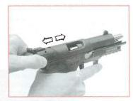
If the slide is already automatically locked into the rearward position after having fixed the last round (also refer to § 4.7), this step is not necessary: Just press the slide release lever dawnwords in order to let the slide return to its forward position.
