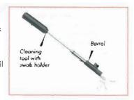
Be careful not to scrotch or damage the muzzle as this can affect occuracy: it is recommended to clean from the rear side.
