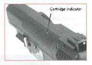
As the hammer of the Five-seveN® IOM pistol is not visible (so that its condition cannot be determined at a glance), ALWAYS consider the pistol as ready-to-fire when the cartridge indicator is protruding and the manual safety is at the (lower) 'fire' position I
