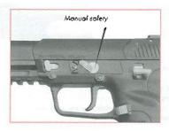
When the manual safety is at the (raised) 'safe' position, the red marks are NOT visible.
