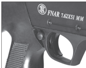
"Safety" shown in the on safe position.
