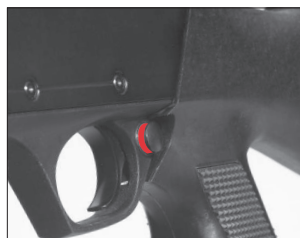
"Safety" shown in the off safe position.
