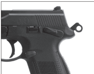
Hammer cocked for single-action firing
