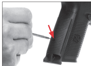
Use a small instrument to press the backstrap retainer.
