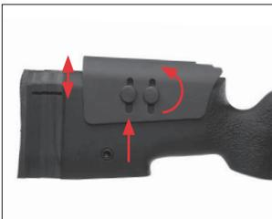
Loosen the locking screws and move the cheek piece up or down. Note its position with the index lines.
