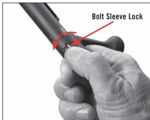
Press the bolt sleeve lock. Unscrew the bolt sleeve.
