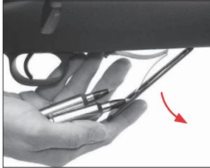
Catch the cartridges as the floorplate swings down.
