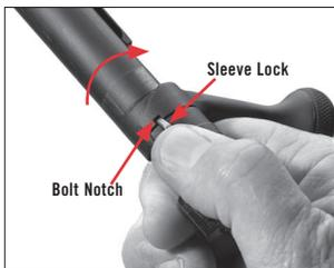
Turn the bolt sleeve. Make sure the sleeve lock is in the bolt notch.
