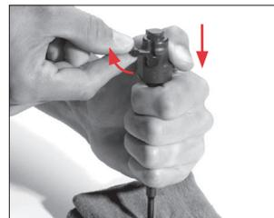
Move the "safety" lever into the intermediate position.
