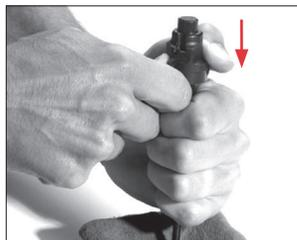
Compress the firing pin spring with your thumb.
