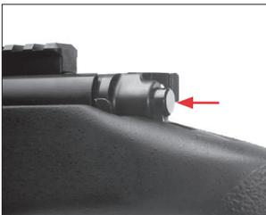
The firing pin indicator (shown cocked).
