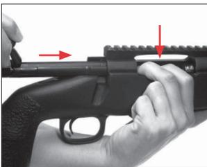
Load the rifle to full capacity by placing a cartridge in the chamber, pressing down the top cartridge and closing the action.
