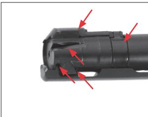
Lubricate the CRF bolt at these locations.
