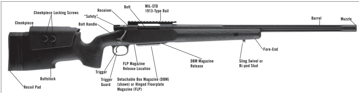
resulting in the rifle firing. During the rearward movement of the bolt, the empty cartridge case is ejected out of the ejection port.
