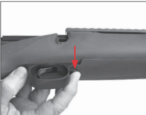
Press the floorplate catch.
