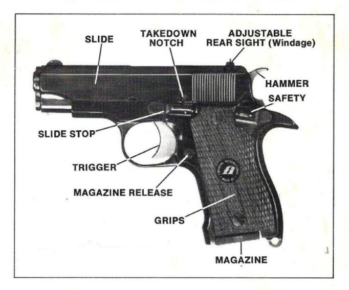
**LOADING:** Each time you pick up the pistol, grasp the serrations on the rear of the slide between your thumb and fore-finger. Draw the slide to the rear and check to be sure the chamber is empty. Even if you just removed the gun from its box for the first time, never assume the gun is empty.
