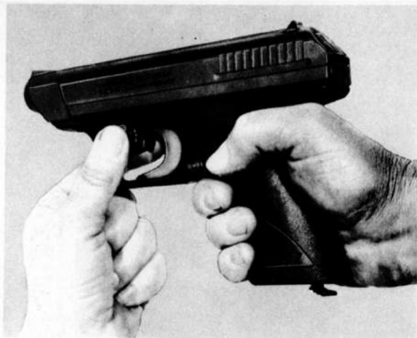
Fig. 6: Pull retaining catch downward
