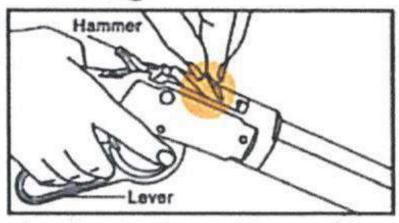
lower edge of cartridge chamber. Push cartridge nose-first down grooved loading ramp, and all the way forward until it is stopped by the ejector. Now close the action by raising lever until breech block raises to top of rifle and locks.
