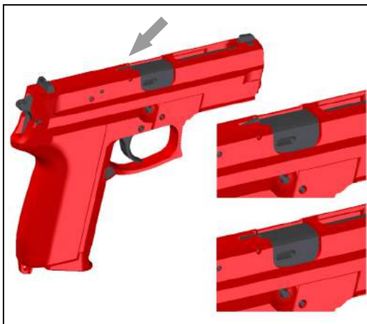
Fig. 2. Load state indicator above: loaded, below: not loaded
