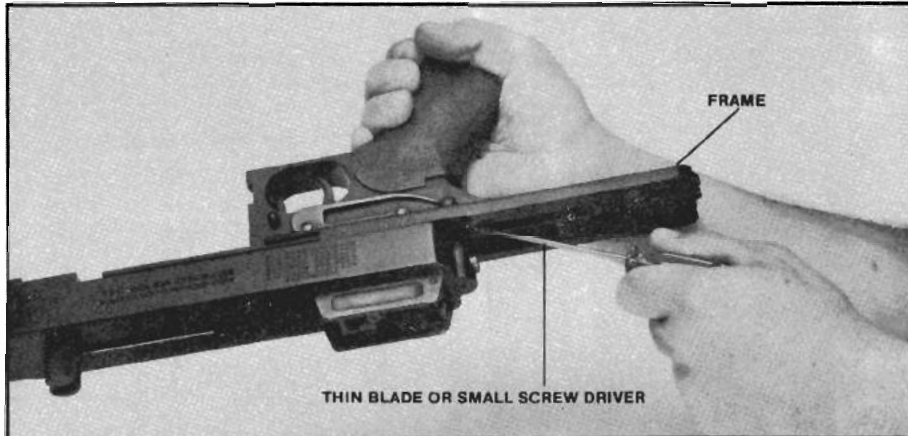
Fig. 2. Depressing frame latch button.
