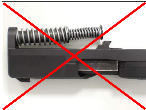
FIGURE 22.3: Spring not seated
