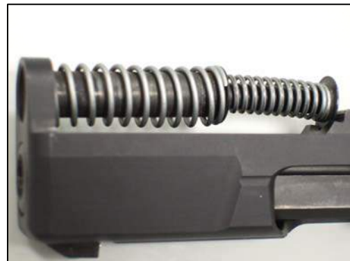
FIGURE 22.4: Spring correctly seated
