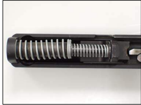
FIGURE 22.2: Spring correctly aligned
