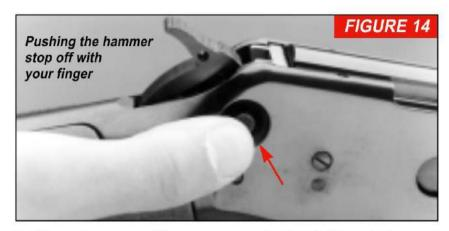
2. Place the manual hammer stop in the "off" position (See Figure 14) by pushing it from right to left.
