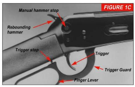
manual hammer stop built into the receiver, as well as our rebounding hammer system. This rifle also contains an automatic hammer stop which blocks the hammer from striking the firing pin until the trigger is pulled. These advanced features move the traditional Model 94 design to a new level of convenience and safety. All features are explained in detail later in this manual.
