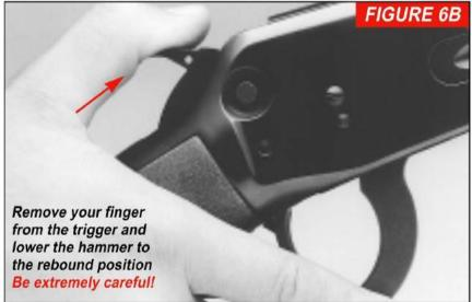
3. While holding the hammer back apply just enough pressure on the trigger and finger lever to release the hammer from the full-cock position. Immediately remove your finger from the trigger and slowly and carefully allow the hammer to lower into the rebound position (See Figure 6-B).
