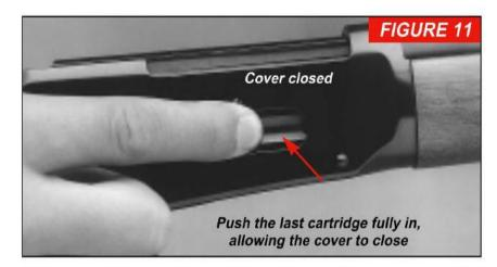
3. Repeat this procedure with each cartridge, but push the last cartridge past the end of the spring cover, allowing the cover to snap closed (See Figure 11). Do not exceed the recommended capacity of the magazine.
