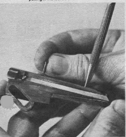
When replacing the pin that retains the takedown screw, note that the pin is slightly smaller at one end, and be sure that this end is inserted in the hole. Grip the pin with sharp-nosed pliers to start it, then tap it into place with a small drift punch and hammer. Remember that the pin must have equal projection on each side of the takedown screw, to allow the screw to move toward the left during takedown and reassembly.
