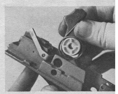
17. Push the hammer pivot out toward either side (left), and remove the hammer assembly upward (right). The hammer spring and its two nylon support pieces are easily removed from the hammer.
