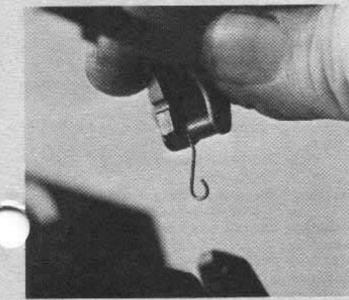
When driving in the firing pin stop pin on the left side of the bolt, insert the bolt handle temporarily to prevent loss of the extractor pivot pin.
