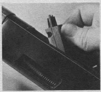
Move the bolt toward the rear to clear its forward end from the barrel throat, and tip the front of the bolt upward (the gun is still inverted) until it can be removed from the receiver. Caution: The bolt spring is under tension. Ease it out.
