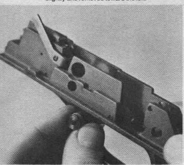
19. Push out the trigger pivot pin, and remove the trigger from the top of the trigger housing. The sear contact stud on the trigger is factory-staked at the proper level, and it should not be disturbed.
