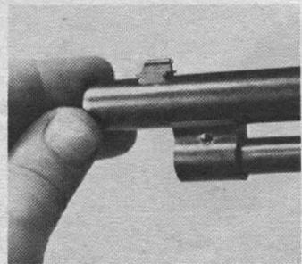
Drifting out the small, short cross-pin in the magazine tube hanger near the muzzle will release the outer magazine tube for removal toward the front. This will allow the fore-end to be taken off downward. After removal of the fore-end, the nylon foreend mount is easily slid out of its dovetail toward either side.
