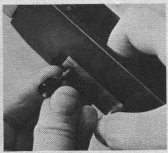
With the gun inverted, retract the bolt slightly and use a finger or tool to hold it inside the receiver. Lift the front of the bolt, and remove the bolt handle from its hole in the bolt.
