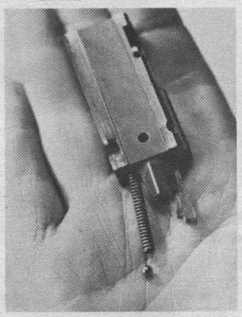
14. Move the firing pin toward the center of the bolt, and remove the firing pin toward the rear.
