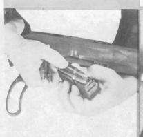
Load magazine with four cartridges.
