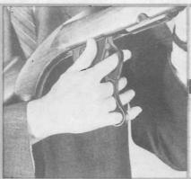
Open and close action by operating lever in order 10 put on SAFETY. (Safety is inoperative unless Hammer is cocked.)
