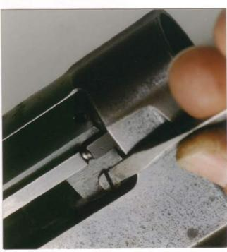
11. Remove the screw on the right side of the bolt just below the extractor. This is a long screw going though the length of the bolt.
