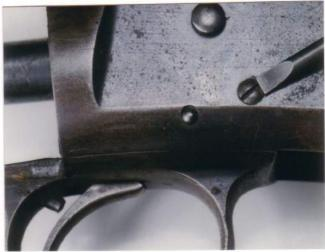
**6.** Remove the small screw on the right side of the receiver, just forward of the
