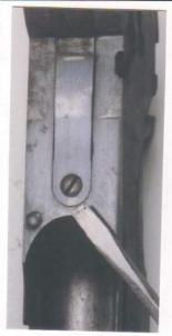
**24.** Remove the sear spring screw on the underside of the carrier, and take off the spring downward.\*\*Read reassembly tip after Step #36.
