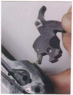
35. Remove the hammer upward. Repairs Only: Do not remove the stirrup.
