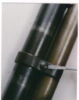
**40.** Remove the screws on each side of the magazine band, and move the band off toward the front. When the band is removed, the screw bushing at the center can be taken out. The action slide and magazine assembly can now be removed toward the front.
