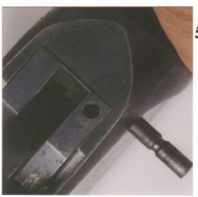
5. Remove the carrier pivot pin toward either side.
