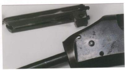
13. Slide the bolt all the way to the rear of the receiver and remove it.
