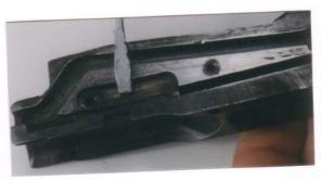
**30.** Remove the action slide lock spring.
