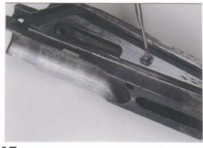
**27.** Remove the slide lock joint pin stop screw.
