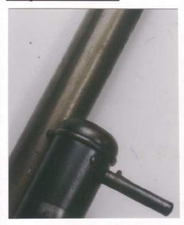
**38.** To remove the magazine lock pin, depress the round wire spring in the slot in its side and pull out the pin.
