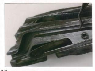
28. Insert a slim drift in the access hole in the lower edge of the action slide track, and push out and remove the slide lock joint pin downward. As the pin emerges, it can be grasped and pulled out.
