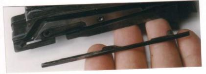
29. Remove the action slide lock bar.
