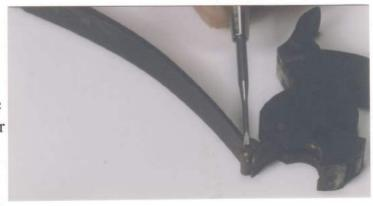
37. Remove for Repairs Only: The shell guide plate is riveted in place on the carrier, and removal is not recommended in normal takedown. If necessary for repair it can be taken off but a new rivet will likely have to be made.
