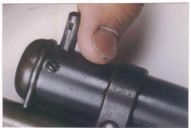
1. Push the magazine locking pin toward the right, and pull it out until it stops. Using the pin as a lever, rotate the magazine tube about one quarter turn counter-clockwise until it stops. Pull the magazine tube up toward the front until it stops.
