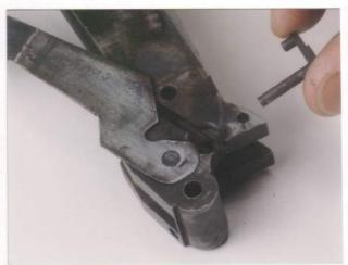
**31.** Swing the shell guide plate upward, and remove the slide lock release plunger toward the right.
