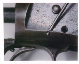
**8.** Cock the hammer, push the carrier release button on the right side, and insert a tool between the bolt and carrier, through the port in the right side of the receiver, to nudge the carrier downward. Remove the carrier downward and toward the front.
