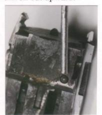
22. The right extractor is removed by inserting a small screwdriver between the extractor and its plunger. Depress the plunger toward the rear, and lift the extractor out of its recess. Keep the plunger under control, slowly release the
