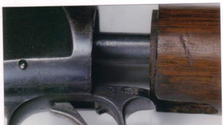
3. Remove the buttplate, and use a stock tool or a long shanked screwdriver to back out the stock bolt. Remove the butt stock toward the rear.
