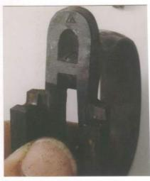
10. The trigger and its spring are easily removed from the top of the guard. The pin was removed in Step # 7. Not recommended for normal takedown: There is also a trigger stop screw at the rear inside of the guard and it is easily backed out. If this is done, though, it will have to be readjusted during reassembly.
