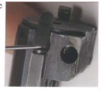
23. Restrain the hammer, and press the tail of the sear upward to release the hammer. Ease the hammer down to its full forward position.
