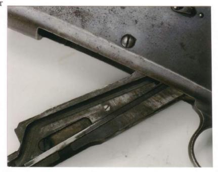
9. Slide (or tap with a non marring hammer) the trigger guard unit out toward the rear.
