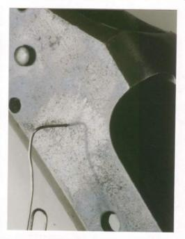
16. The carrier release button is retained inside the receiver by a round wire spring, that is keyed into a tiny hole in the receiver wall. Use a tool of very small diameter to push the tip of the spring inward, then use a pair of sharp nosed pliers inside the receiver to move the spring forward, releasing the button for removal. \*Note for replacement.
