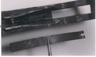
**36.** Nudge the mainspring toward the rear. When it has cleared the front bridge of the carrier, the spring can be removed upward.
