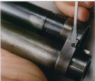
engagement with the teeth on the edge of the sleeve. Turning the sleeve counter clockwise will tighten the barrel engagement. Adjust in small increments. If necessary the screw sleeve and lock piece can be removed (clockwise).
