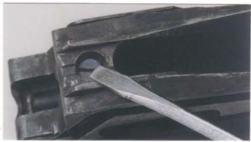
**32.** Remove the mainspring tension screw.
