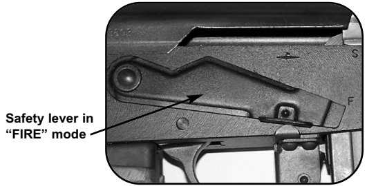
Safety lever in lower or "FIRE" position. Pulling the trigger when the safety lever is in the lower position will result in the rifle firing if there is a round in the chamber! Exercise extreme caution when handling rifle in this condition.
