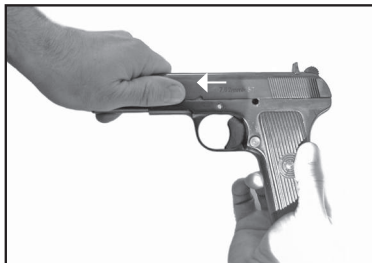
Fig. 8> Separating the slide
