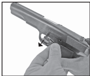
Fig. 7> Taking out the coupling
