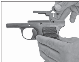
Fig. 9> Separating the trigger mechanism from the frame
