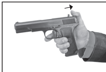
Fig. 4> Blocking the trigger with the hammer lowered
