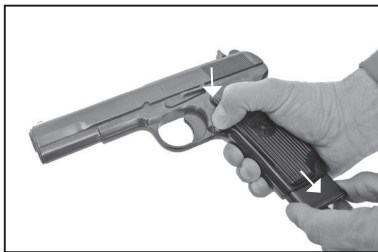
Fig. 5> Taking out the magazine
