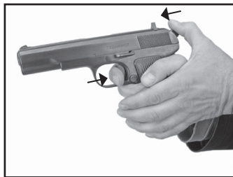
Fig. 3> Blocking the trigger with the hammer cocked
