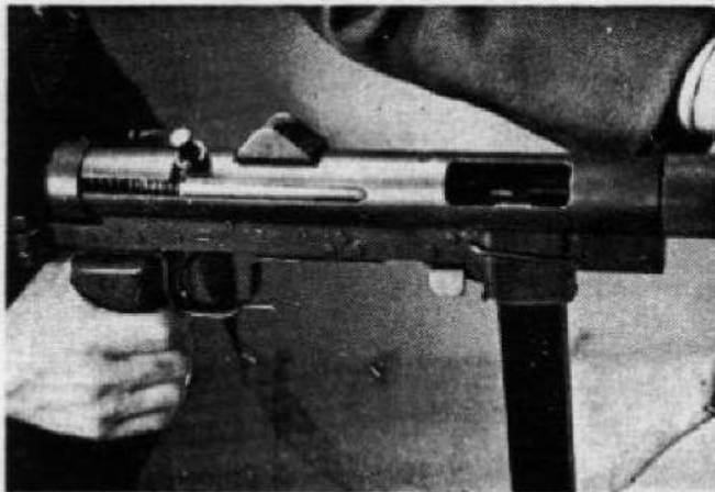
Fig 6. The gun is made safe. Notice that the cocking handle is in the safety slot.
