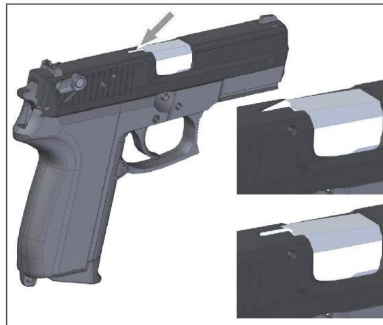
Fig. 3, Load state indicator top: loaded, bottom: unloaded,
