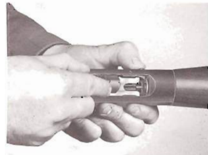
To load next shell keep carrier lock button depressed and repeat step 1.
