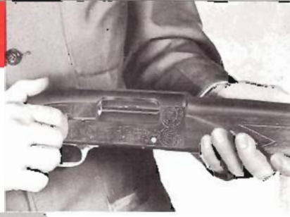
Grip cocking piece and pull bolt back until bolt latches.
