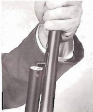
3 Apply firm downward pressure and twist barrel one quarter turn until threaded holes in magazine tube and barrel lug line up.
