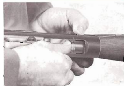
Depress carrier lock button, press shell down on carrier and insert into magazine. Be sure head of shell passes end of carrier lock. (KEEP BUTTON DEPRESSED). The shell will then remain in the magazine while the next shell is being loaded.
