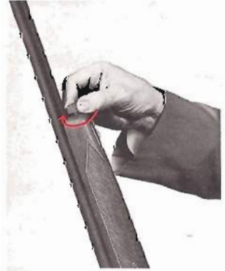
5 Tighten take-down screw in clockwise direction.
