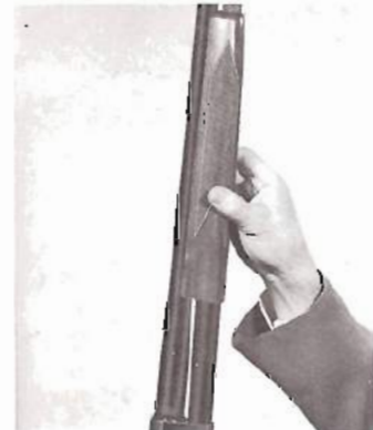
4 Replace forearm on magazine tube and seat against receiver. Take-down screw will enter hole in barrel lug.
