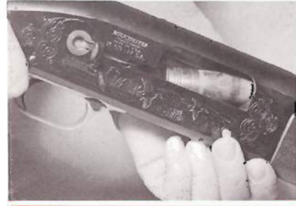
Depress carrier lock button. This releases bolt and loads shell into chamber.
