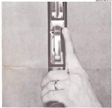
Put on safety by pushing button from left to right until red band disappears.
