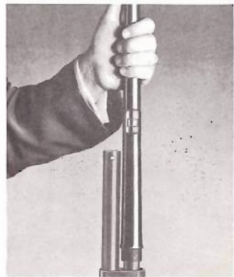
2 Align grooves on barrel shank with non-grooved areas in receiver.
